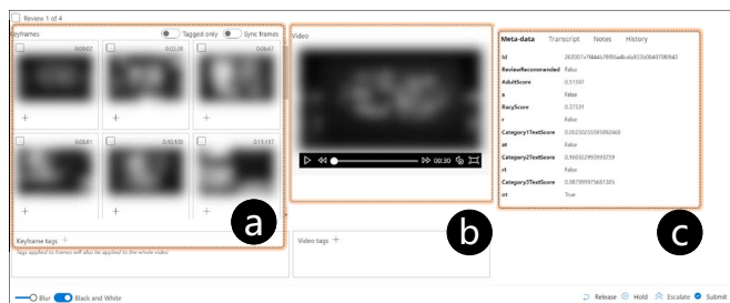
Fig. 7. ContentModerator [3] consists of (a) small multiples to visualize video frames, (b) a player to browse both video and audio content, and (c) a form view presenting meta-data and risk information.
